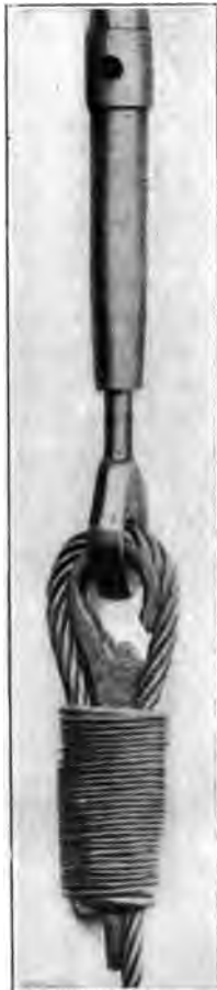
FIG. 18. UNSOLDERED FIELD TERMINAL FOR AVIATOR STRAND.
